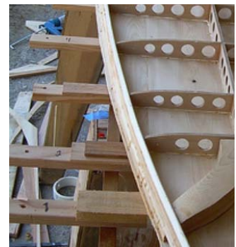
FIGURE C-4. (right) Keel blocks support the frame.
