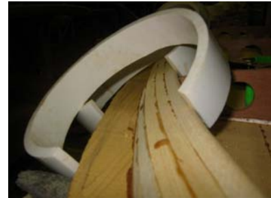
FIGURE C-5. Clamp applied to railstrip. This clamp should have a drilled hole making a half-moon divit in each of the edges right where they bear on the bottom planks and the railstrip bead.
