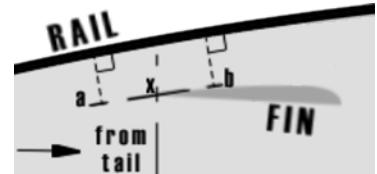
FIGURE B-3. Initial reference point for trailing edge location - 'x' marks the spot..
